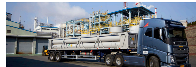
Tube trailer high-pressure hydrogen tank
